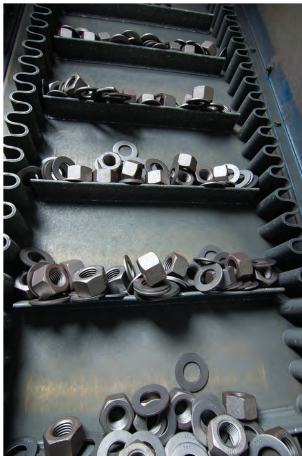
Uncoated fasteners are carried up to the large dip spin basket through a conveyor.
